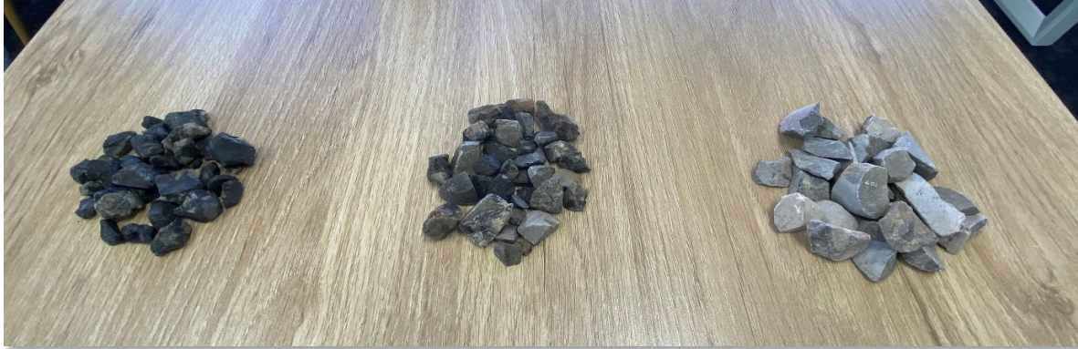
Figure 16: The three products produced from the ore sorting test work. Left to right – Very High Density product (DSO), High Density product, and Low Density product (waste rock)
