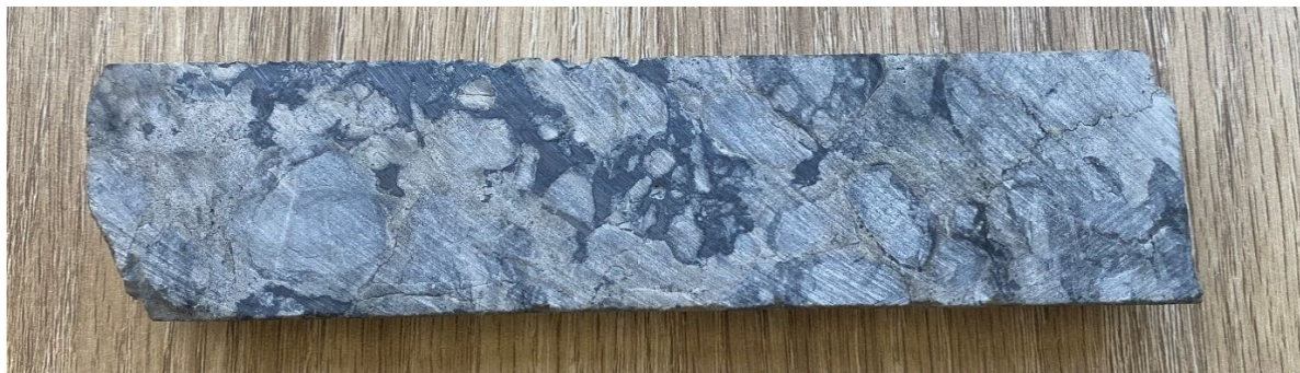
Figure 15: Drill core from STOR1601D from interval 97-101m downhole – average grade 4.16%. The Chalcocite is seen as the dark gunmetal grey material within the lighter grey dolomite host rock.
